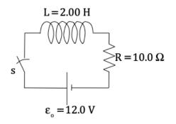
32.16) (This is going to be fun.) At t = 0, the switch in the circuit shown to the right is closed. Labeling the initial and final values for the current, and using a single axes, sketch the *current versus time* graph for  $t \ge 0$ , assuming that:
